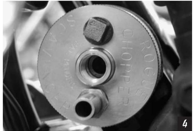
5. Install supplied hose onto hose barb and secure with wire tie. Place open end of hose into suitable empty container.
