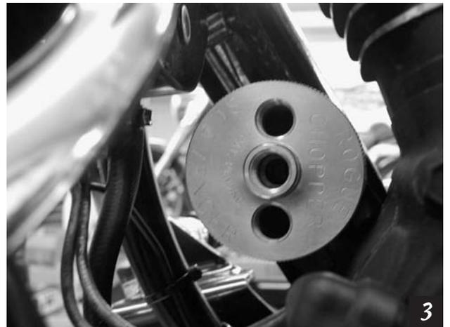
4. Install supplied hose barb fitting in the bottom hole and snug. Install supplied plug fitting in opposite outside hole and snug, leaving center hole open.
